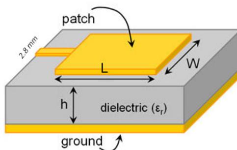
Figure 2. Design of Rectangular Micro-Strip Patch Antenna at 2.2 GHz
