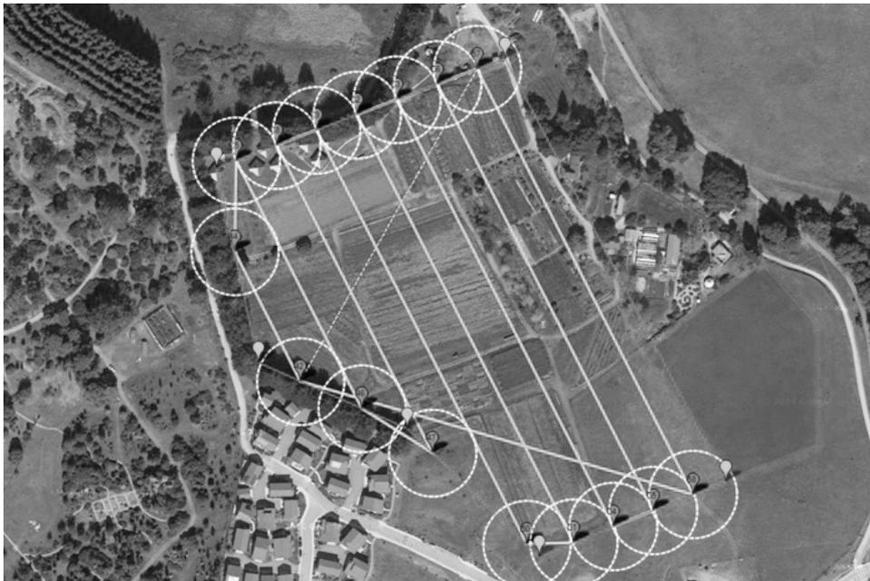
Figure 1. Edge detection of green field using multispectral camera and setting the trajectory of quadcopter.
