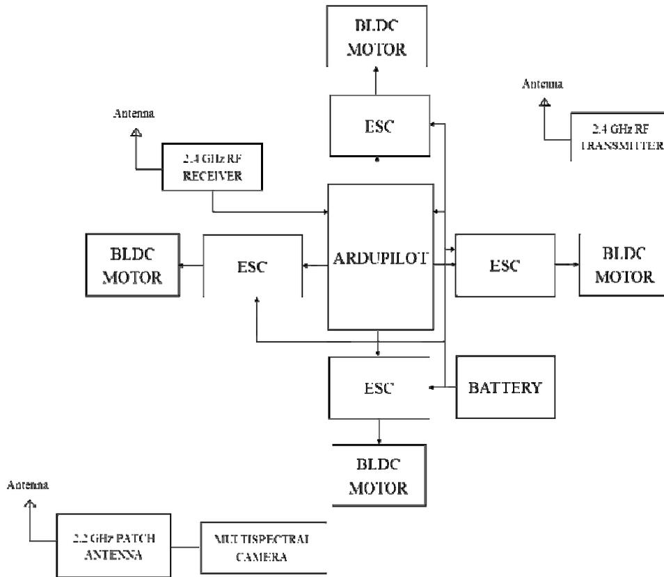
Figure 3. Block diagram of quadcopter. This figure shows the blocks incorporated in the design of quadcopter.
