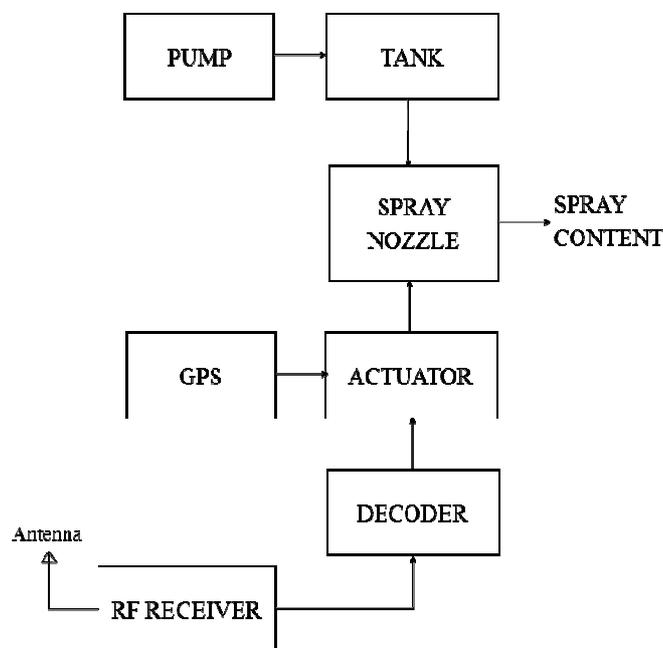
Figure 4. Block diagram of Sprayer Module. This figure shows the blocks incorporated in the design of sprayer module. The sprayer module is integrated into the quadcopter.
